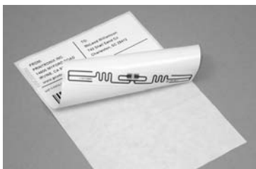
A microchip and a flexible antenna, which form a tag, are placed in a plastic inlay and embedded in a shipping label to make a smart label.
